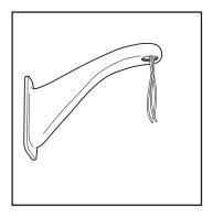
a. Install the mount for the pendant dome. Refer to the instructions supplied with the mount. Bring the wiring for the dome through the mount. Refer to Tables A and B in the Appendix for wiring distances.
